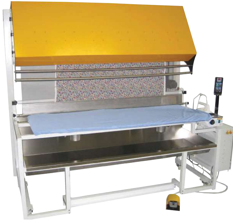
Drying machine based on infra-red technology
