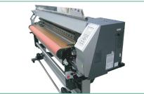
The system invented and patented by Top Digitex is used in thousands of printers worldwide. The system is based on a series of cylinders that move the fabric (or the substrate in general) under the printer head. It offers an economical, speedy and user-friendly solution. Machine specifications can be defined based on the required dimensions, speed, and drying capacity.
