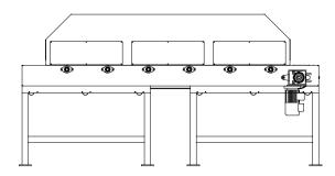
Top Digitex drying systems are based on infrared technology and could be dimensioned on customer request. The infrared technology consists on lamps or panels with different thermal inertia and irradiation power. Machine characteristics can be defined based on dimensions, speed and drying capacity required.
